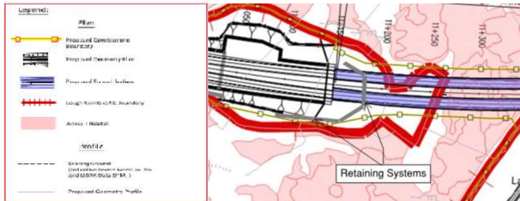
Figure 5.13: Lough Corrib cSAC Pinch Point between Ch. 11+150 and Ch. 11+180
